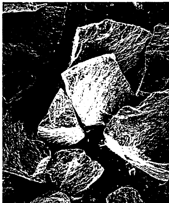
Fig. 1. Scanning electron micrograph of 50% graphite PFC particles. The individual particles are irregular in shape and exhibit characteristic dimensions in the range 74–149 \mu\text{m} .
